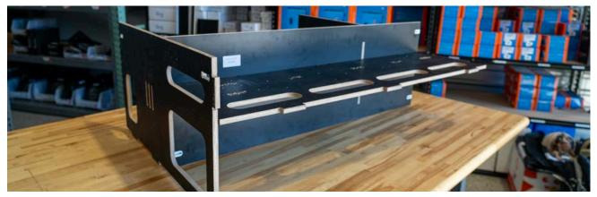
Attach Bottom to Component Panel and Vertical Divider using 4 wishbone connections (non-textured side down). Use rubber mallet to tap into place
