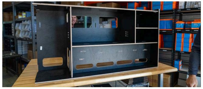
Simultaneously attach Left End Panel, Upper Fuse Panel Brace, and Lower Fuse Panel Brace to the Bottom Panel and Top Panel using tongue and groove connections.
