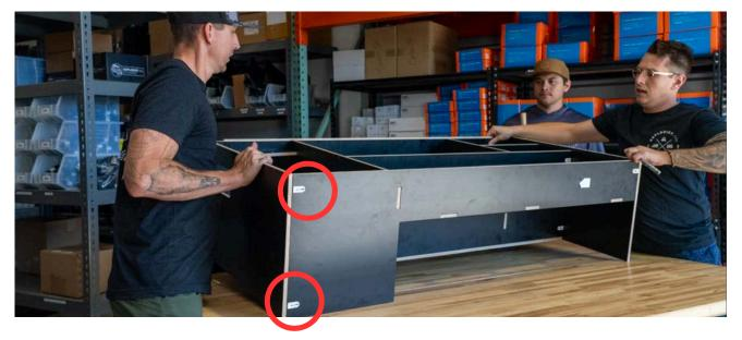
Tighten screws (2) on Bottom Panel into Left End Panel
